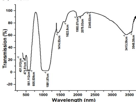
**Fig. 3: FTIR analysis of microbial synthesized hydroxyapatite by *Klebsiella* sp PSM7.**
