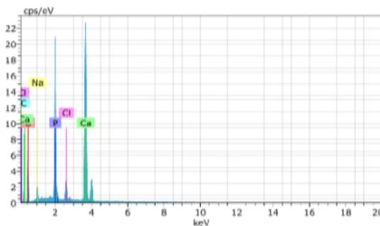
**Fig. 6: EDX profile showing the Ca and P signal of hydroxyapatite powder.**
