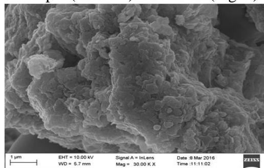
**Fig. 5: FESEM image showing irregular spherical structure of hydroxyapatite synthesized by *Klebsiella* sp PSM7**
