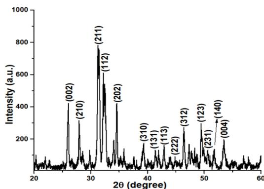
**Fig. 4: XRD pattern of the *Klebsiella* sp PSM7 synthesized hydroxyapatite**
