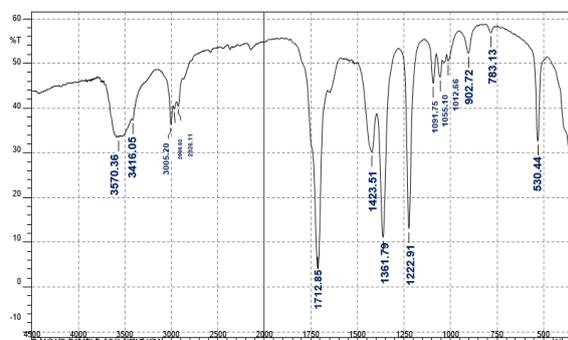
Fig 4. FTIR spectra silver nanoparticles synthesized using *A. cepa* leaf extract with 1mM silver nitrate solution
