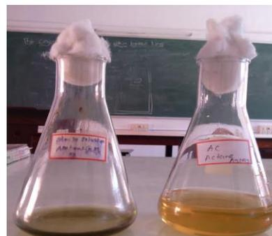
Fig.2. Colour change during the bioreduction of AgNO<sub>3</sub> into AgNPs using plant extract: before synthesis (left) and after synthesis (right).
