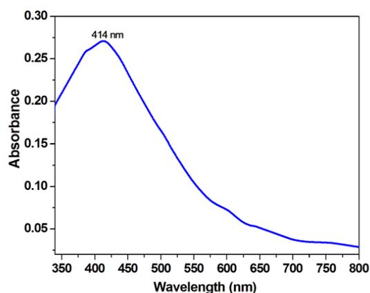
Fig 3. UV-Vis spectra of silver nanoparticles synthesized by treating *Allium cepa* leaf extract with 1mM silver nitrate solution.
