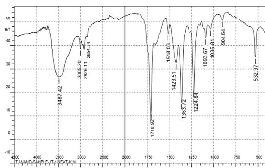
Fig.4: FTIR spectrum of biosynthesized AgNPs
