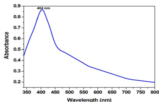
Fig. 3: UV-Vis spectra of silver nanoparticles synthesized by treating *Achyranthes aspera* leaf extract with 1mM silver nitrate solution.
