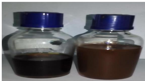
Fig.2: Colour change during the bioreduction of AgNO<sub>3</sub> into AgNPs using plant extract: before synthesis (left) and after synthesis (right).
